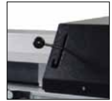
Lever to lift the rollers up and down
